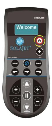
LCD SCREEN - Indicates when the SolaJet is powered "On" (displays time remaining) or "Off" (displays "welcome" once the track has reset at the foot end of the bed). When adjusting the various functions, the controller displays the selected setting and then returns to time left. Do not press multiple functions at one time and always wait for screen message to exit before selecting next function.
